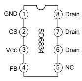
Note: it is Decommended to connect pin 5 to pin Drain for better heat dissipation.
